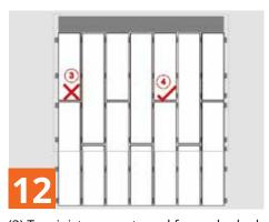
(3) Two joists are not used for each plank at the jointure.
