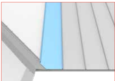
Place the sheet in the gully and push in the folded edges around the folding board and the valley gutter's fastening device.
