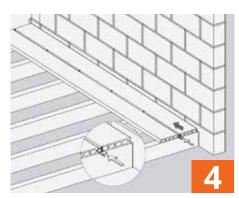
Take your next decking board and securely push into the universal clips. Nip the screw to secure.
