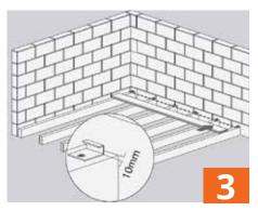
The first decking board should be secured with starter clips and thereafter use one universal clip and screw on every joist. Do not screw or nail through the decking board and do not overtighten at this point.
