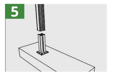
Place the aluminum post onto the steel holder.
