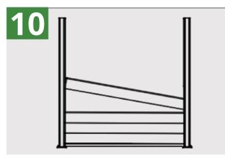
Slide the boards one by one between the posts. Note that the slats fit on top of each other so that the boards are fitted perfectly in place.
