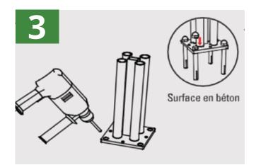
Position the plate of the steel holder, then drill some pilot holes using a drill bit with a diameter of Ø12mm, and fix the plate with the screws provided.
