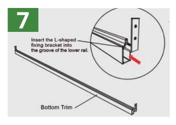
Remove the L-bracket from the bottom trim. Insert it according to the drawing above.
