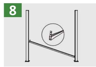
Put the bottom trim kit into the aluminum post groove.
