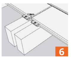
Two independent joists are required where boards ends meet with a 30mm gap provided between the joists. A 5-7mm expansion gap should be allowed between the board ends.
