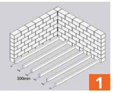
We recommend using 50 x 100mm treated timber joists at centres of 300mm with a minimum of a 1% fall to help water naturally disperse.
