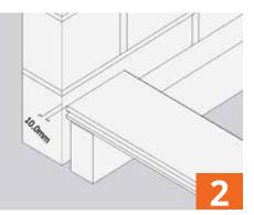
Secure starter clips in line with the joists. It is critical that a perimeter expansion gap of at least 10mm is provided between the decking and the wall and any other fixed objects. Ensure the boards do not overhang the joist at the edge by more than 25mm.
