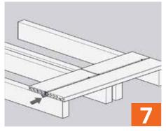
Fit the final boards by first measuring the width of the final two boards to determine where the outer edge of the final board will lie. Mark these areas. Using these marks for starter clips and slot the final board into place. Now insert the penultimate board, slide down the required number of universal clips and fix these into place.
