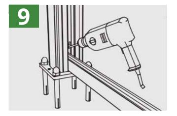
Put the bottom trim between the posts and fix it with screws (M4x19 screw).
