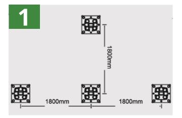
The fence distance between two posts is 1800mm. The fencing board can be installed lengthwise, in "L" or in "T".
