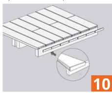
If using end caps, push the end caps into the exposed hollow board ends. We recommend applying a small amount of a High Grab External Adhesive to the end caps for extra adhesion. Wipe away any excess from the edge of the cap.
