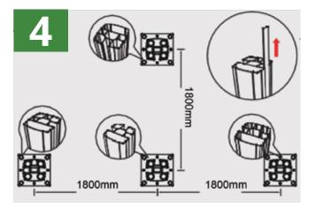
Each post kit has grooves on two sides with strip bands, which are removable to match the different types of installation desired.
