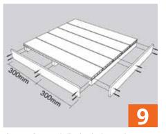
If using fascia, drill pilot holes with counterbore through the fascia at 300mm intervals. According to ambient temperature allow a minimum of a 5mm expansion gap between the end of the deck board and the fascia. Screw fascia to the joists. Always screw fascia to the joist at a 90° degree angle.
