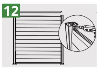
Position the top trim between the posts and screw it into position.
