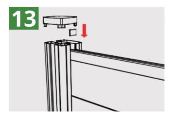
Insert the small finishing piece and then cover the post with the plastic cap.
