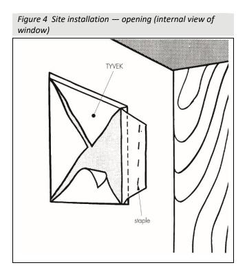
13.5 Nails should be of galvanized or sherardized mild steel, austenitic stainless steel, phosphor bronze or silicon bronze. Staples should be of austenitic stainless steel.
