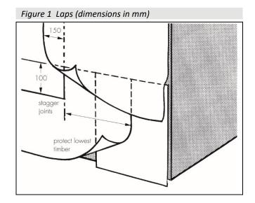
13.3 To assist in achieving the design air permeability, the lap joints and penetrations through the product can be sealed with TYVEK 2060B Tape or TYVEK 1310D Tape.
