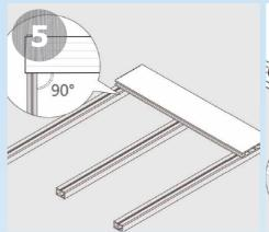
Put first decking planks on vertical way of joists, fasten the first plank by Starting Clips at outside of decking. The position and direction of first plank should be accurate guaranteed to be the reference for the following planks.
