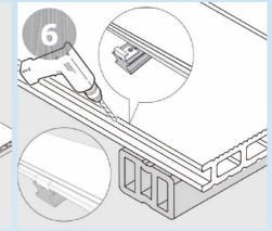
First plank should be fasten by Starting Clips.
