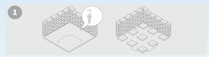
Punching holes  $\Phi$  6 in the installation area with impact drill. Recommended width ways and lengthways distance between two holes is 350mm. Knock the plastic expansion pipe  $\Phi$  6 into the holes and make sure it is tight enough and will not expose.
