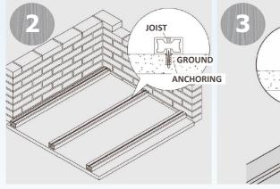
Take expansion pipes as centre line and lay the joists (cut if necessary) on the line. Dr ill corresponding holes in the joists and fix the screws into the expansion pipes through the holes.
