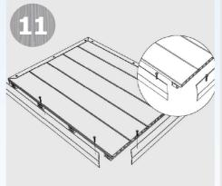
Fasten the finishing strip with screws.
