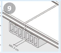
In case of the deformation caused by temperature change, joists should not be too tightly connected. We recommend the distance between two joists is 3cm.
