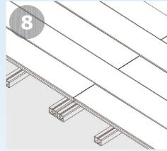
Two joists are needed for each plank at the jointure.
