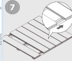
Place the Stainless steel clips in the right position and screw it. Insert the second plank into the clips then repeat this process.
