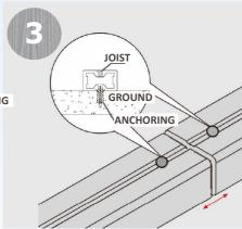
Extra fixing of expansion blots are necessary on both joists near juncture. The holes should be at least 3cm to the end of joist.
