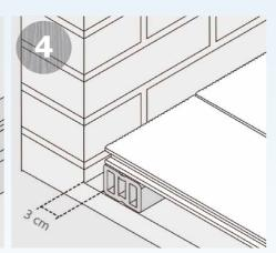
Allowing for the expansion and maintenance, sufficient distance around your terrace and by obstructions such as walls, fences, trees, etc. should be at least 3cm.
