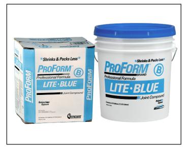
If Lite-Blue Joint Compound freezes, allow material to thaw at room temperature for at least 24 hours. When thawed, turn the container upside-down for at least 15 minutes. Turn pail right side up, remove lid and immediately remix with an electric drill. Lite-Blue should be lump-free and ready to use within 1 minute. Discard all joint compound that does not remix to a lumpfree consistency.
