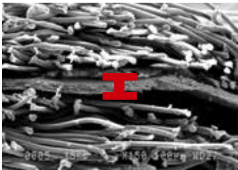
Standard multilayer Membrane: 30 microns (internally measured)
