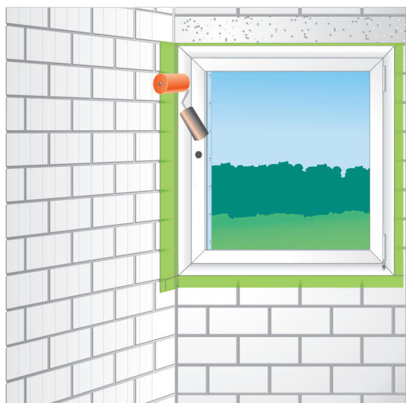
illbruck ME501 bonded to face of window frame and wall with SP525 adhesive
