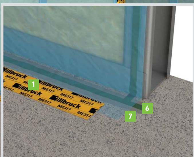
Floor to wall interface detail
