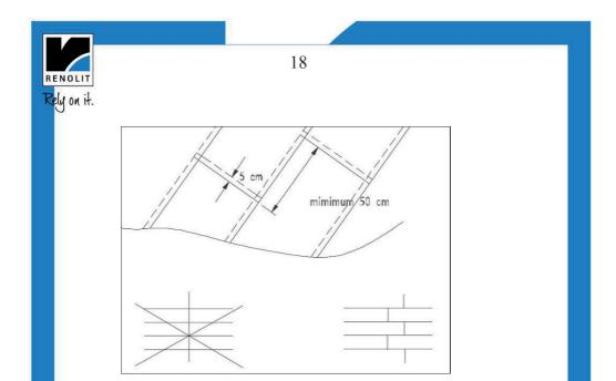
End laps from the end of the roll of **RENOLIT** ALKORPLAN roofing membrane must be cleaned to remove any tape or adhesive used in the rolling of the membrane and then must be overlapped by 50 mm and welded in the normal way. The end joints across the roof must be staggered to give a minimum of 500 mm between each joint.
