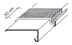
Followed by a 200 mm wide junction strip of **RENOLIT** ALKORPLAN D (unreinforced) or ALKORPLAN F reinforced membrane welded to the metal strips with a 35 mm effective weld width.
