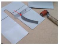
this. Any tears must be located outside the welded joint, or in the area of the reinforcement.
