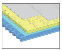
fasteners and washer tubes or plates.
