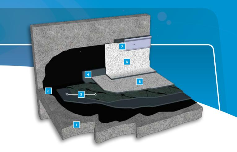
In this case the waterproofing element is applied fully adhering to the support, using a hot air or a propane gas torch. This type of application favours better puncture resistance and can be used on any pitch.
