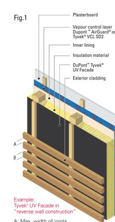
A: Max. width of joints B: Min. width of facade elements  $B \ge 2A$
