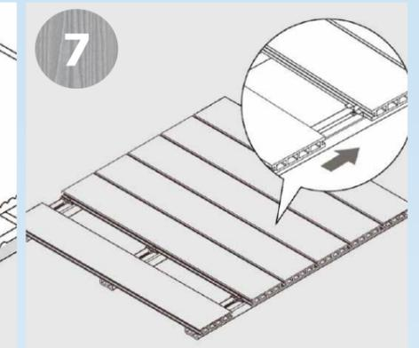
Place the Stainless steel clips in the right position and screw it. Insert the second plank into the clips then repeat this process.
