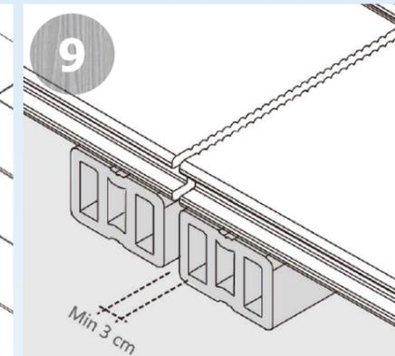
In case of the deformation caused by temperature change, joists should not be too tightly connected. We recommend the distance between two joists is 3cm.
