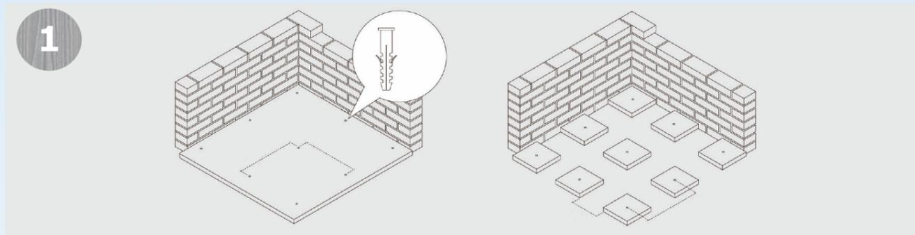
Punching holes  $\Phi 6$  in the installation area with impact drill. Recommended width ways and lengthways distance between two holes is 350mm. Knock the plastic expansion pipe  $\Phi 6$  into the holes and make sure it is tight enough and will not expose.
