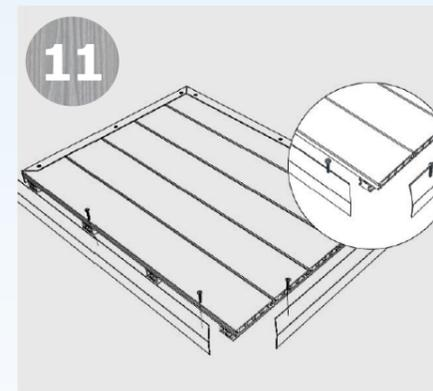
Fasten the finishing strip with screws.
