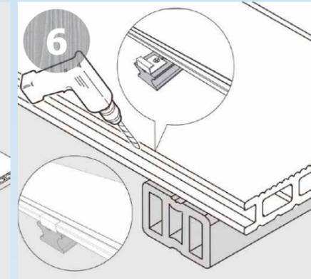
First plank should be fasten by Starting Clips.
