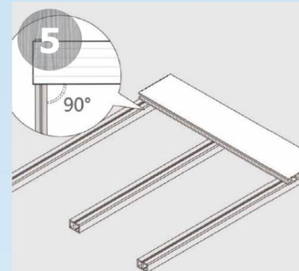
Put first decking planks on vertical way of joists, fasten the first plank by Starting Clips at outside of decking. The position and direction of first plank should be accurate guaranteed to be the reference for the following planks.
