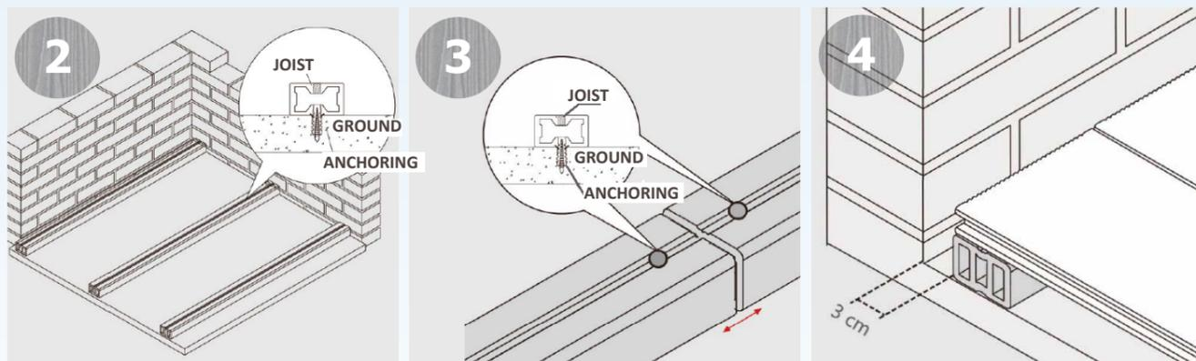
Take expansion pipes as centre line and lay the joists (cut if necessary) on the line. Drill corresponding holes in the joists and fix the screws into the expansion pipes through the holes.
