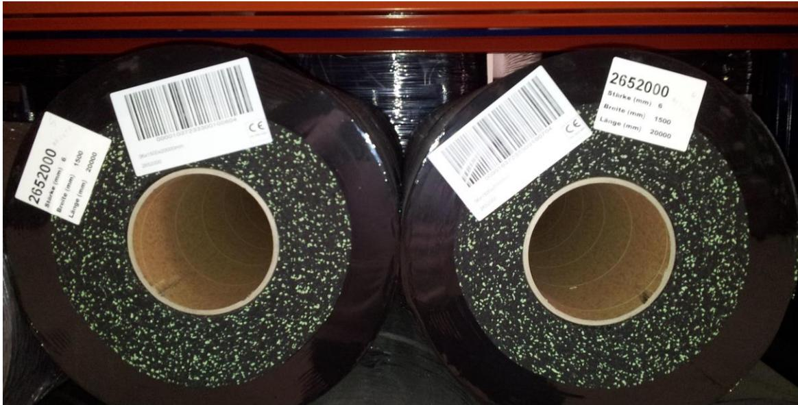
**Figure 4:** Pay attention to the production batch reference, placed with labels on the rolls
